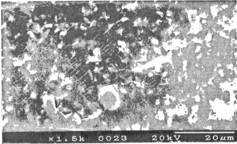
FIGURE 10d DENS micrograph ( 20^{\circ}\text{C} , 500\text{ mm}\cdot\text{mm}^{-1} ) showing slight particle-matrix debonding and matrix shear yielding.
